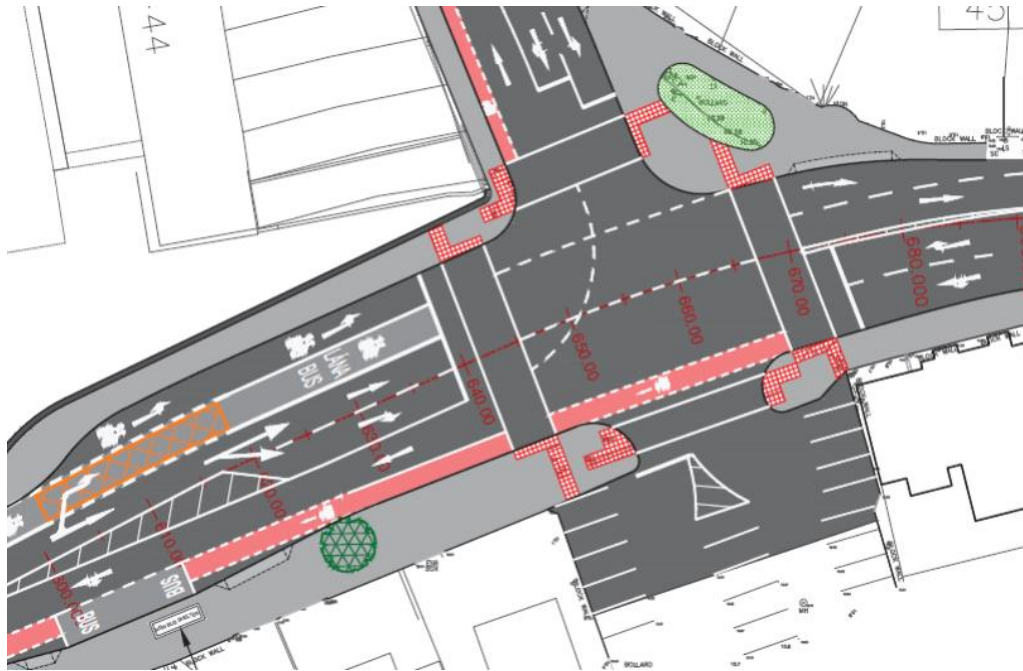
Figure 28 Skehard Road/Church Road Proposed Junction Upgrade Layout
